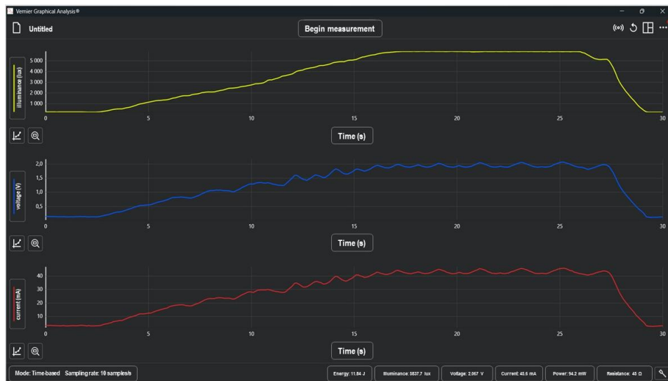
Figure 7: Graph showing the relationship between illuminance, voltage, and current
